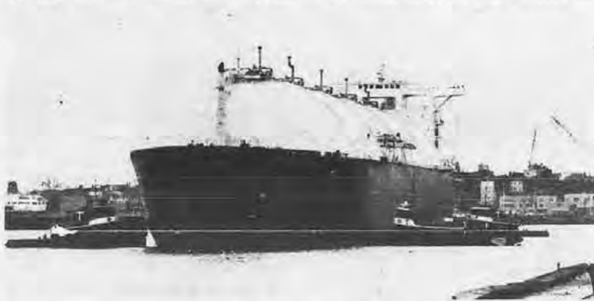
The imposing Aquarius , with her five spherical cargo tanks towering above her deck is ushered through Boston harbor by regiment of tugs.
