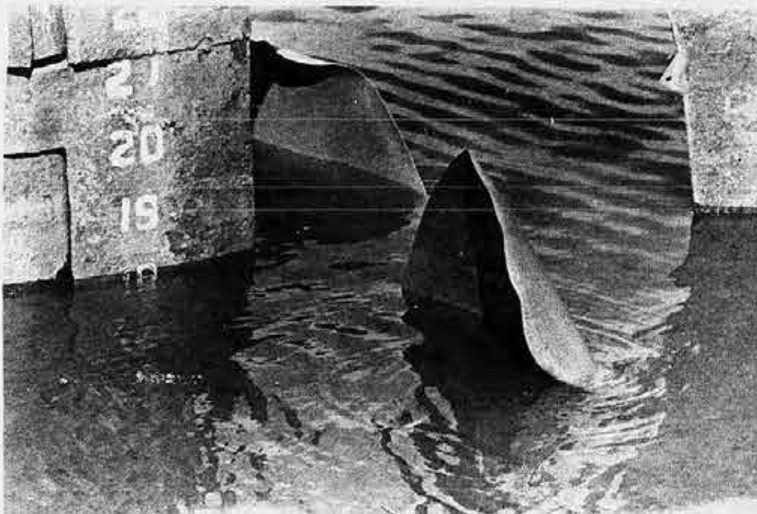
Looking somewhat like the fins of an angry shark, the bent propeller blades on the Steel Voyager resulted from a run-in with a submerged obstacle. A short stopover in the shipyard put propeller in shipshape condition again.
