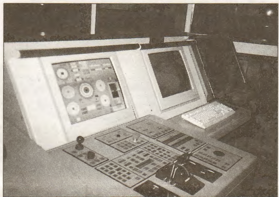
Seafarers at the Paul Hall Center last month raved about the bridge simulator, which includes a 360-degree viewing sector and provides teaching support in GMDSS (among many other areas). It also is interactive with an auxiliary bridge.
