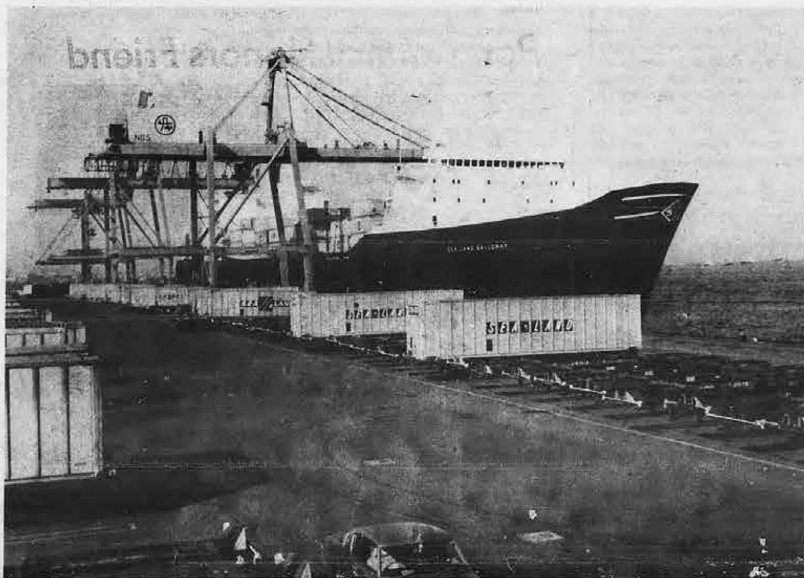
The SL-7 Sea-Land Galloway unloads containers at the Sea-Land dock in Yokohama. SL-7s are 946-foot long and carry 1,094 containers at a speed of up to 33 knots.
