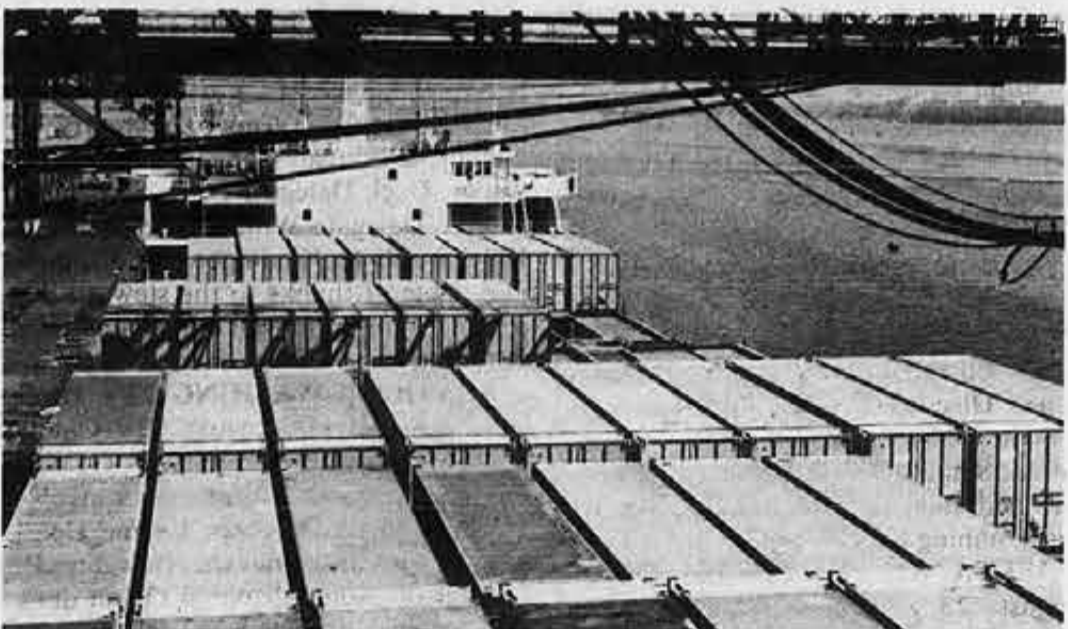
Looking forward from the Sea-Land Resource's stern, the photographer's wide angle lens captures a small portion of the SL-7's 1,094 container cargo. Above is part of the huge crane used to unload the containers.
