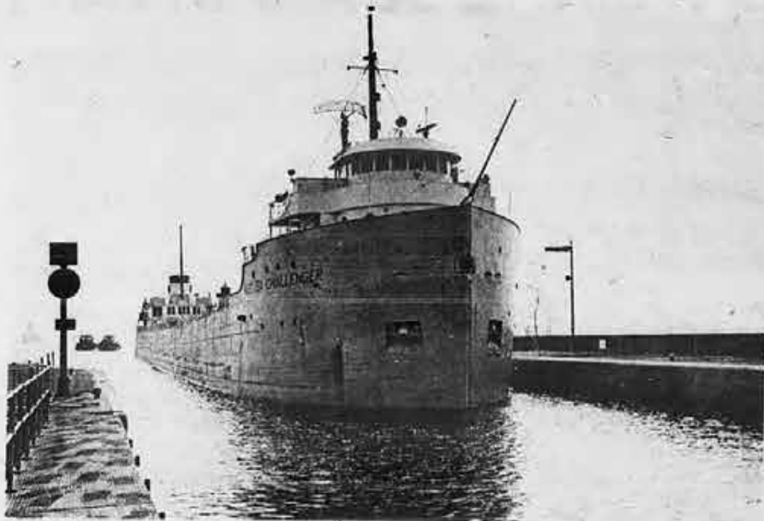
This SIU-contracted Great Lakes freighter, the Medusa Challenger (Cement Transport), gets ready to enter a lock. As is common on most Great Lakes ships, the pilot house is directly in back of the bow, while the crews quarters are placed far aft.
