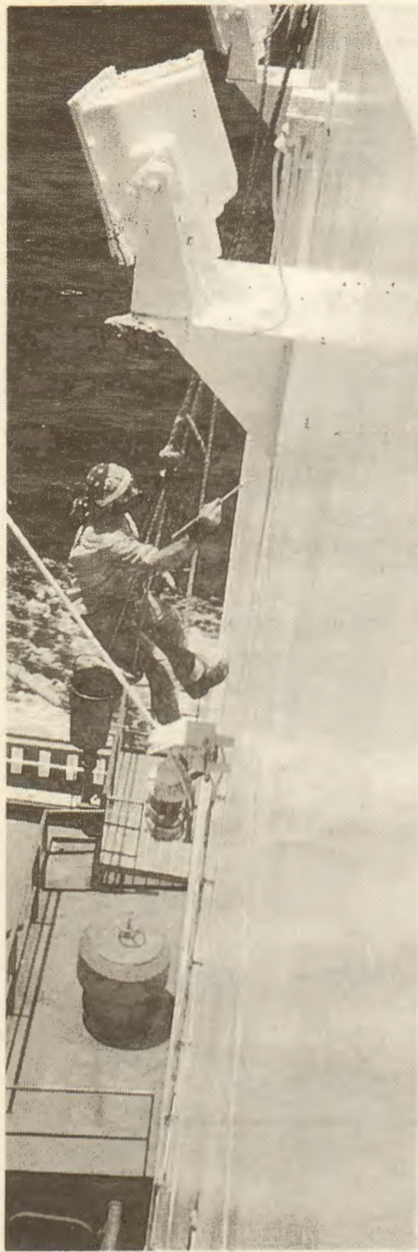
AB Bruce Collins cuts in draft numbers while suspended in a bosun's chair high above the main deck of the Gus Damell .
