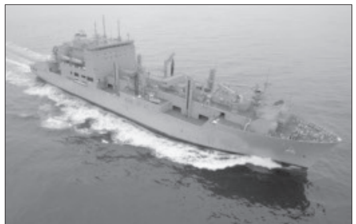
The USNS Lewis and Clark (above), the first ship in the T-AKE class, completed sea trials April 25-29 off the San Diego coast and is slated for delivery to the U.S. Navy's Military Sealift Command by the end of June. Crewed by members of the SIU Government Services Division, the Lewis and Clark is a dry cargo and ammunition ship. It is 689 feet long, has a beam of 106 feet and can sail at 20 knots. The vessel was built at the National Steel and Shipbuilding Company yard in San Diego.
