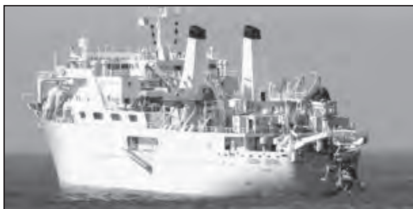
This file photo of the ship (by Todd Walsh) shows the Global Sentinel launching a plow that's used to bury cable beneath the sea floor's surface.
