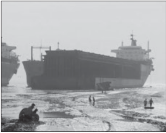
This is one part of a shipbreaking location off the coast of Bangladesh. Ships are beached at high tide so poorly treated workers can take them apart.
