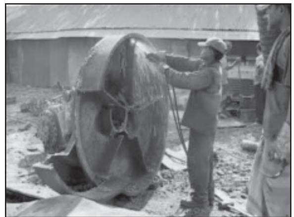
Lacking protective gear, a worker uses a cutting torch to assist in shipbreaking in Bangladesh.
