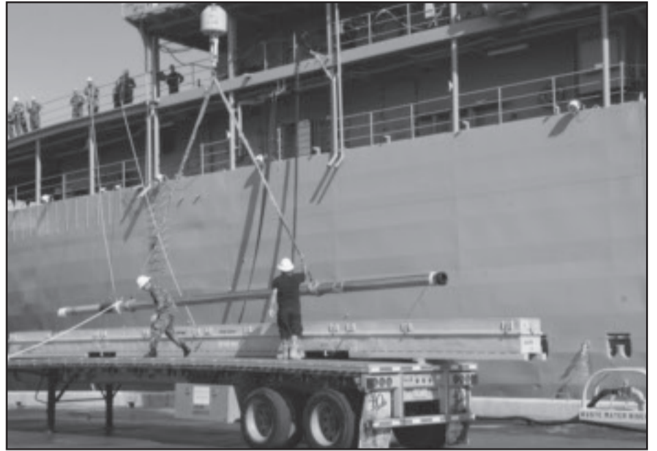
Sailors and Military Sealift Command personnel assigned to the submarine tender USS Emory S. Land hoist a submarine periscope from the pier in Santa Rita, Guam to be loaded onto the ship. This evolution renewed a capability that has not been employed for nearly a decade. Submarine tenders stocked with vital spare parts, such as a periscope, are a key aspect of providing repair support to submarines and keeping them fully operational. (U.S. Navy photo by Mass Communication Specialist Seaman Austin Ingram)
