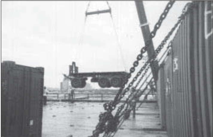
A trailer is loaded by crane onto the Westward Venture .
