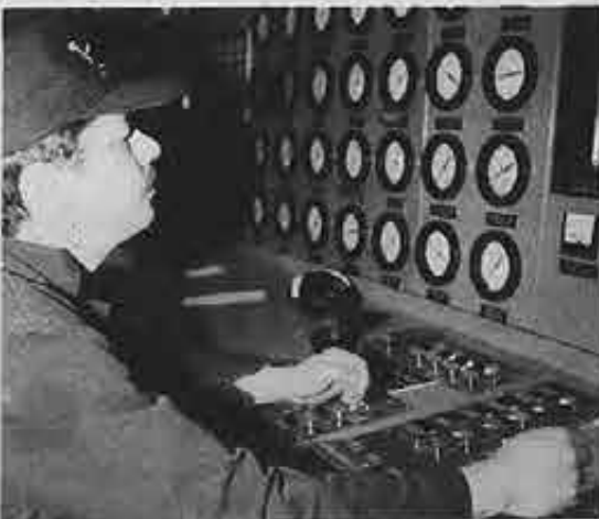
QMED Dave Cameron keeps his eyes on the American Republic engine room control board.
