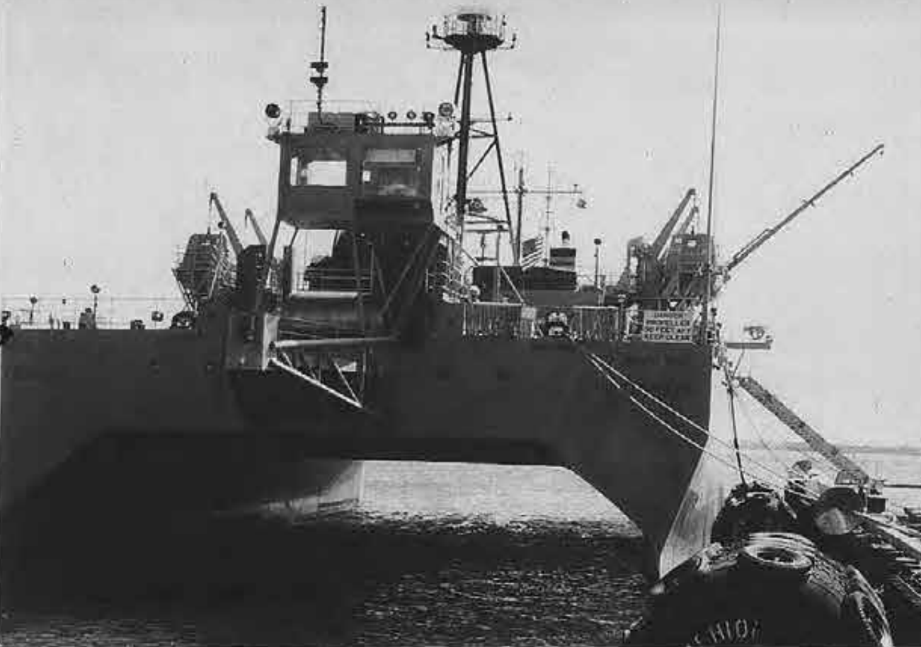
The unique SWATH hull of the USNS Victorious was designed to sustain rough conditions at sea.
