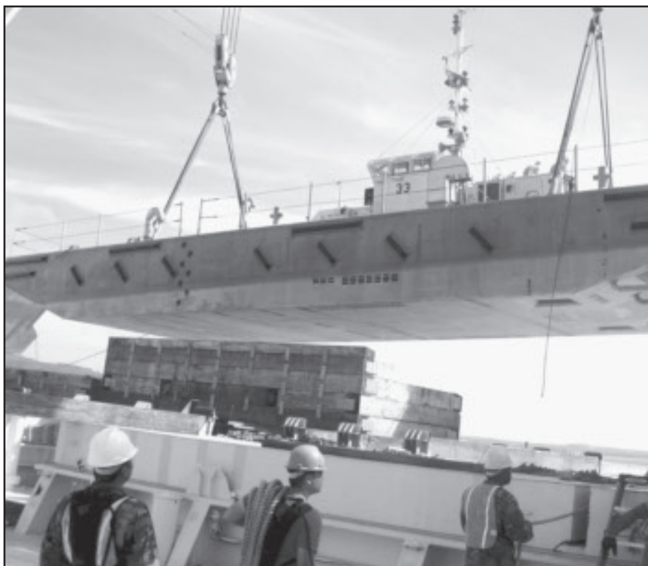
Navy cargo handlers operate the shipboard crane aboard the Lummus to lift an Improved Navy Lighterage System (INLS) power module into the water. The INLS is a floating system designed to offload combat equipment and supplies where conventional port facilities may be damaged, inadequate or nonexistent. (U.S. Navy Photo)
