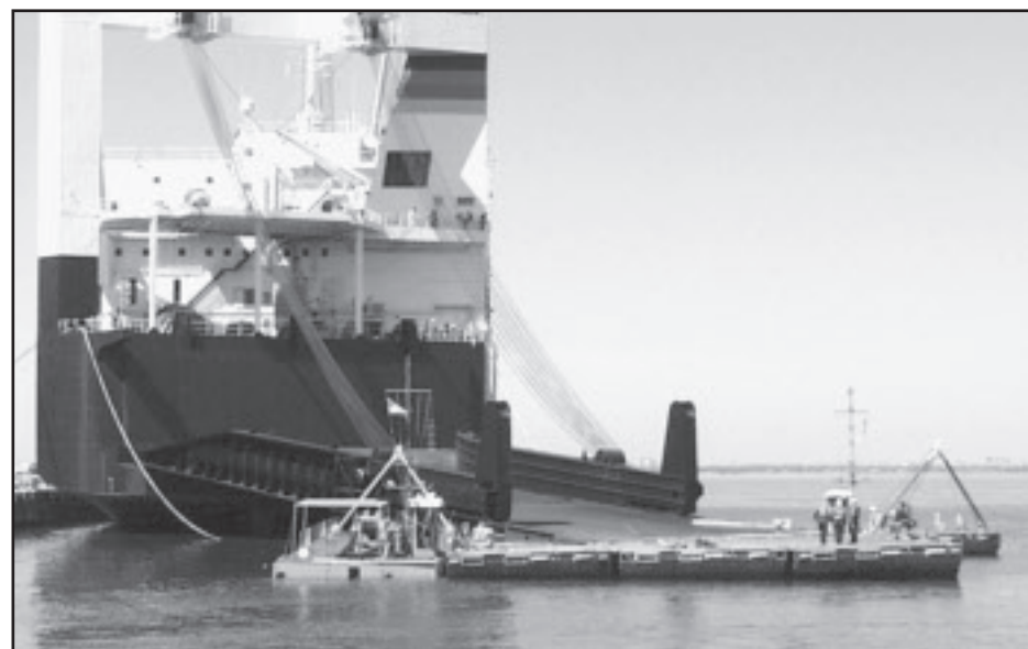
The jumbo stern ramp of the 1st Lt. Harry L. Martin touches down on a roll-on/roll-off discharge facility during Cobra Gold. (Photo by Rick Caldwell)
