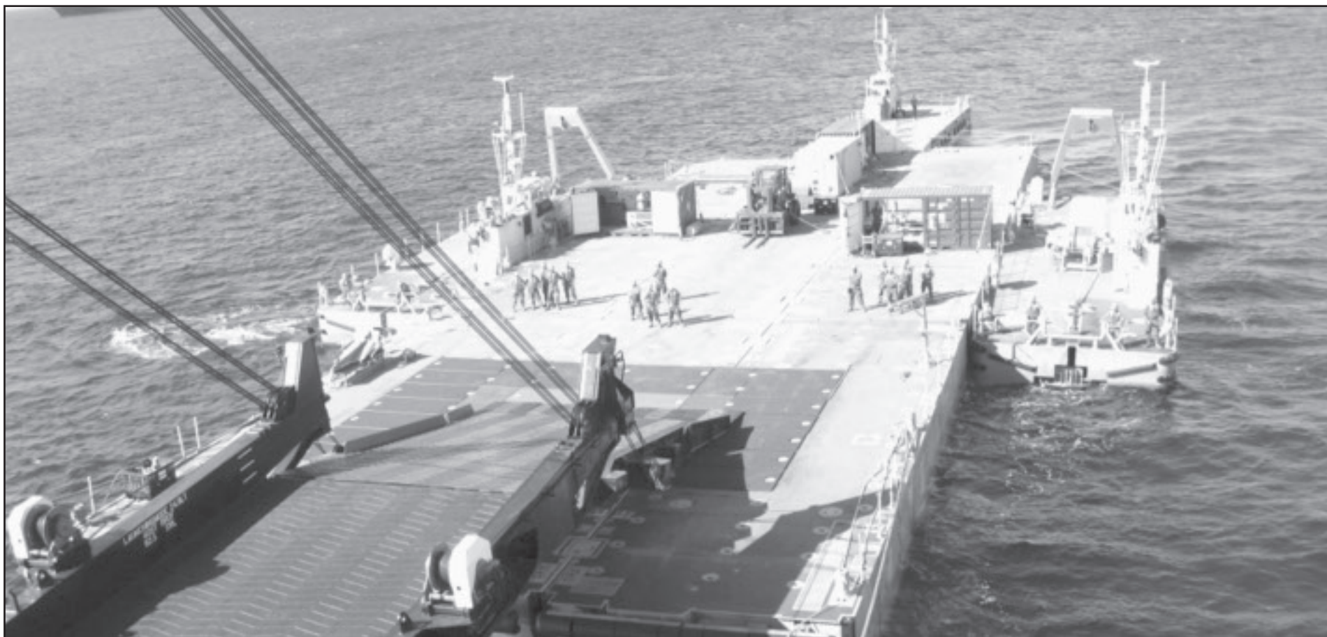
The stern ramp of the Lummus is lowered to the roll-on/roll-off discharge facility (RRDF). During Cobra Gold, this maneuver provided instream offload capability for equipment and supplies. (U.S. Navy Photo)
