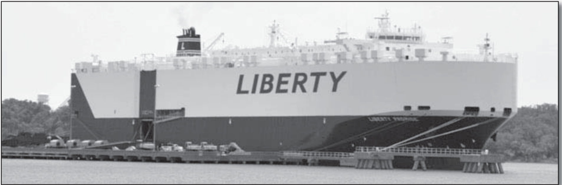
The Liberty Promise can carry up to 6,500 cars and/or Department of Defense equipment such as tanks, helicopters, HUMVEES and MRAPS. Put another way, it can carry approximately enough cargo to fill eight football fields.
