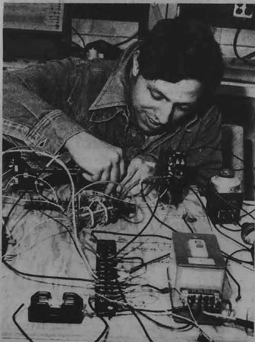
Seafarer Glenn Hutton gets hands-on experience assembling an AC motor control. Seafarer Hutton ships out of the Port of San Francisco.
