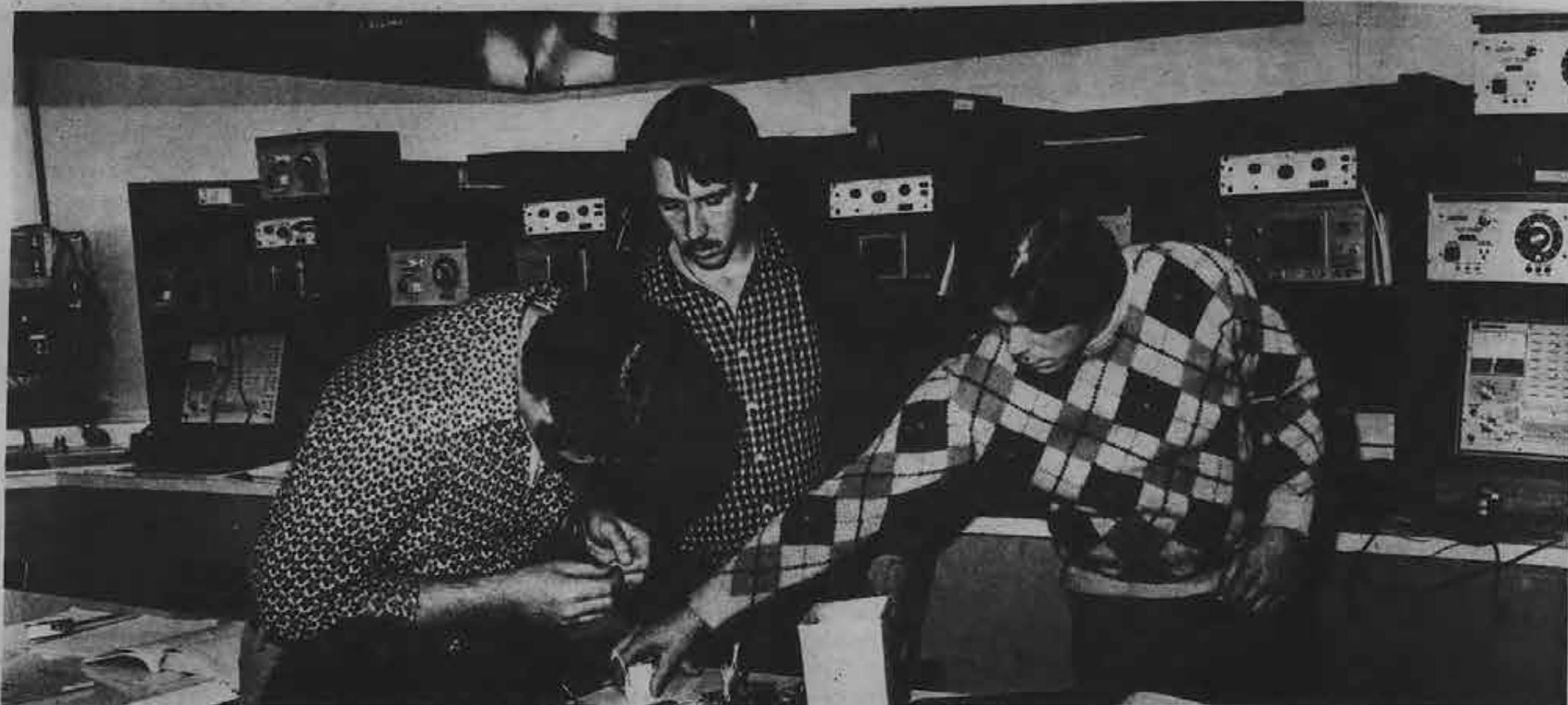
Seafarers David Shaw and Bill Epps work with SHLSS Instructor Jim Harrison in assembling a full-wave rectifier. Seated is Seafarer Mike Murphy. The six-week Marine Electronics course provides both classroom and hands-on training in all phases of shipboard electronics repair and maintenance.
