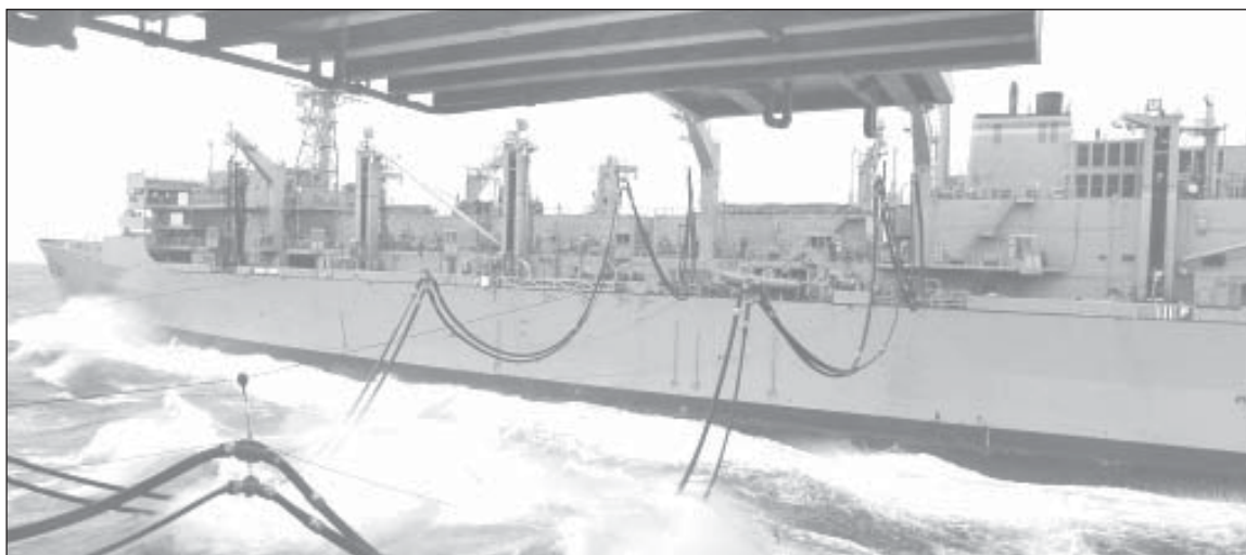
Photo courtesy MSC Fueling hoses from the fast combat support ship USNS Rainier cross rough waters to refuel aircraft carrier USS John C. Stennis during the biennial Rim of the Pacific exercise earlier this year off the coast of Hawaii.
