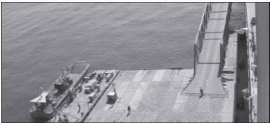
The USNS Soderman's side port ramp (right portion of photo above) is deployed so that an RRDF, the barge-like floating dock in the foreground, could be used during the training exercise.
