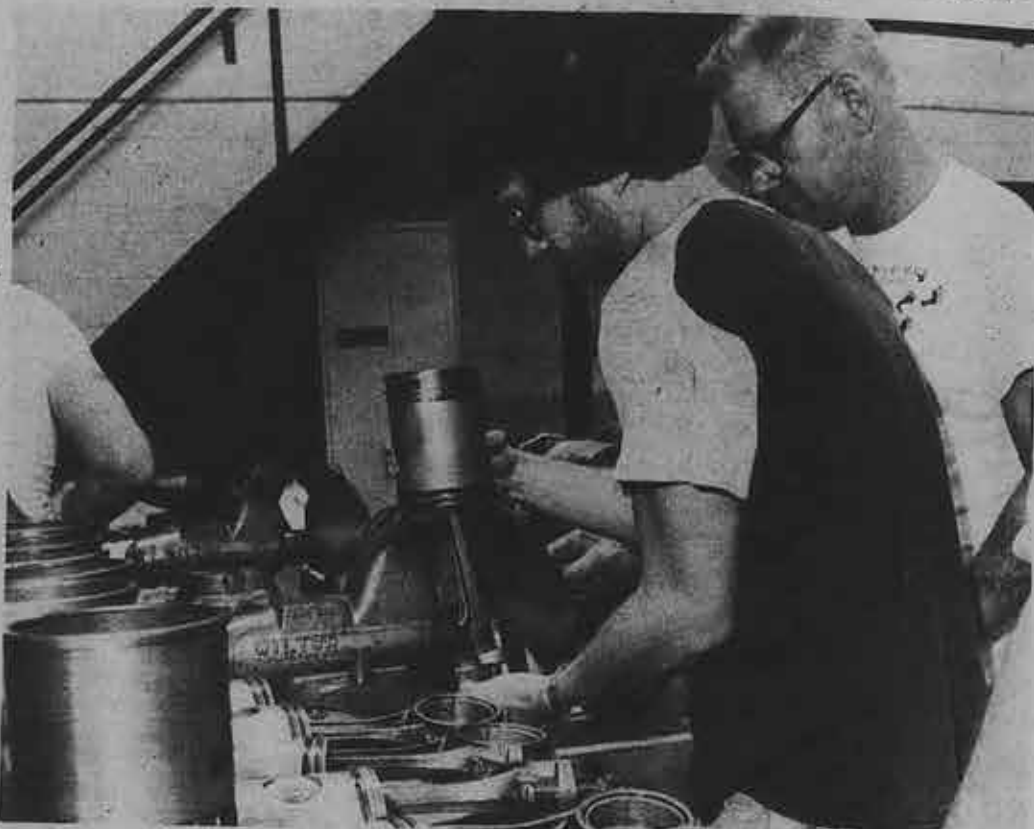
Seafarers Robert Hyams and James Dillon are both in the T.I. Scholarship Program, and both sail out of the Port of Houston. Here, they clean a piston prior to reassembling a diesel engine.
