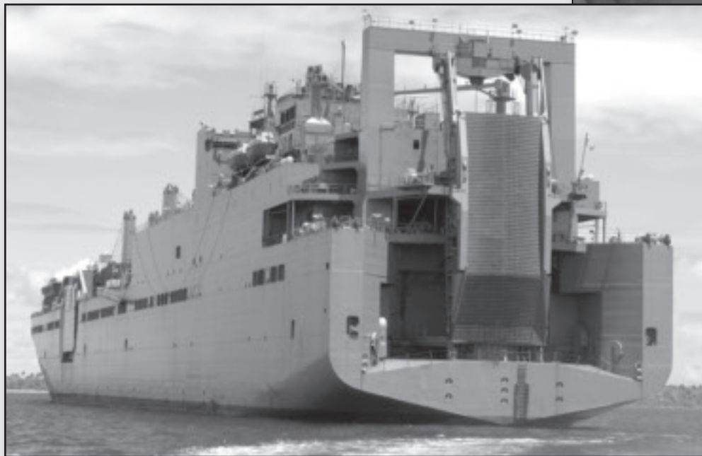
Deploying the vessel's stern ramp makes it easy to drive vehicles on and off the ship.
