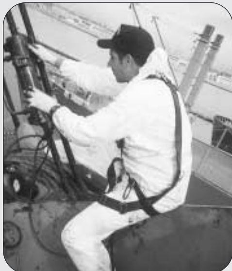
SLUSHING — Cleaning and lubricating the wires (slushing) takes place on a regular basis. Deck department members took advantage of their port time in San Francisco to get some of the work done, as on the Keystone State (above). Performing the task are (below, from left) AB Gheorghe Savencu on the Keystone State , AB Mike Carvalho on the Grand Canyon State and AB John Young on the Gem State . These are three of the Military Sealift Command's 10 crane ships.
