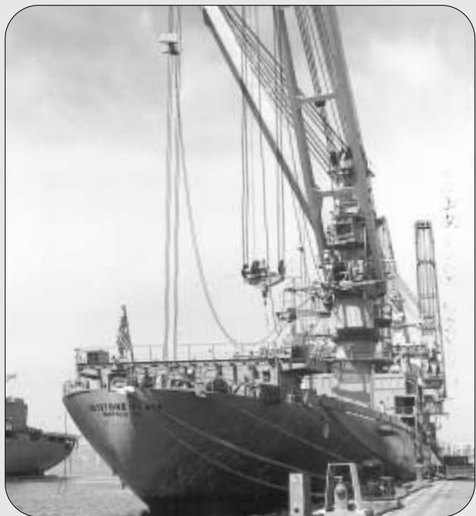
SLUSHING — Cleaning and lubricating the wires (slushing) takes place on a regular basis. Deck department members took advantage of their port time in San Francisco to get some of the work done, as on the Keystone State (above). Performing the task are (below, from left) AB Gheorghe Savencu on the Keystone State , AB Mike Carvalho on the Grand Canyon State and AB John Young on the Gem State . These are three of the Military Sealift Command's 10 crane ships.
