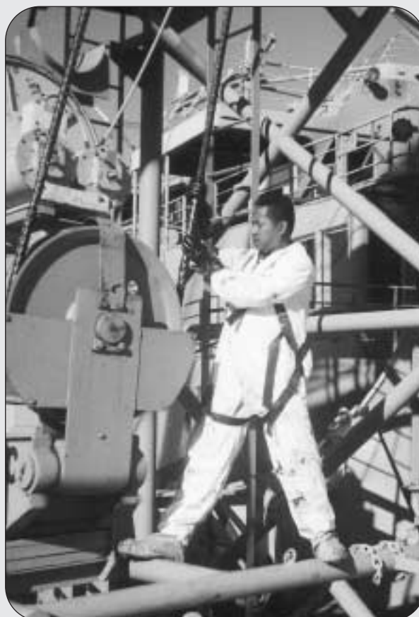
SLUSHING — Cleaning and lubricating the wires (slushing) takes place on a regular basis. Deck department members took advantage of their port time in San Francisco to get some of the work done, as on the Keystone State (above). Performing the task are (below, from left) AB Gheorghe Savencu on the Keystone State , AB Mike Carvalho on the Grand Canyon State and AB John Young on the Gem State . These are three of the Military Sealift Command's 10 crane ships.
