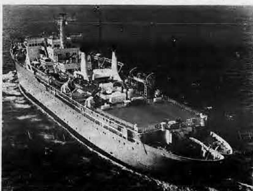
The most modern cable ship afloat, the SIU-contracted C.S. Long Lines pays out deep-sea cable through the stern chute while traveling at speeds up to eight knots in the waters of the Caribbean.
