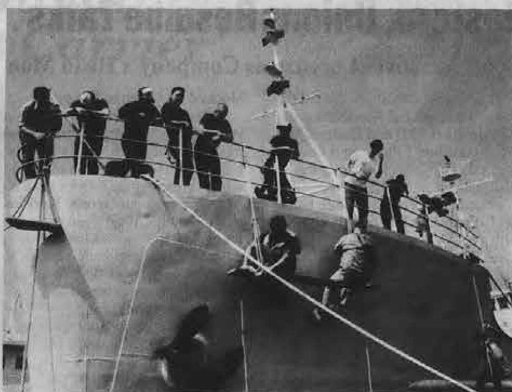
As trainees watch, bosuns go over the side of the Bull Shepard in a bosun's chair to demonstrate safety techniques while chipping and painting.
