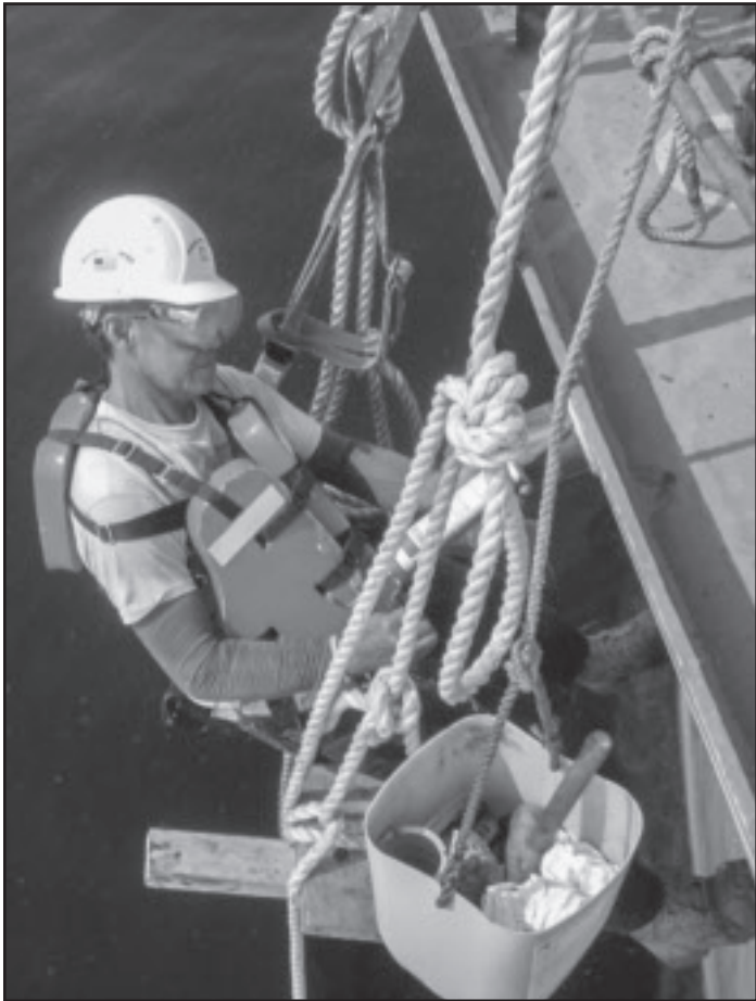
Bosun Gregorio Cudal chips and paints the main deck drain hole.
