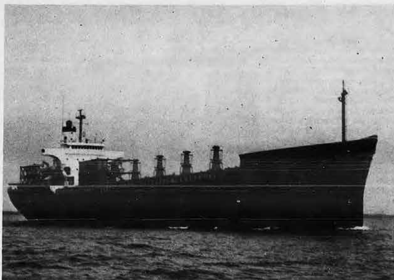
A former troopship, the Philadelphia, now a 20,295-ton containership converted for the SIU-contracted Sea-Land Service, heads for a trial run. Conversion included gutting the mid-ship hull section, removing the mid-ship house, and modifying and enlarging the aft house to provide new living quarters for the crew. The superstructure deck was removed and eight A-frame buttresses installed for containers.
