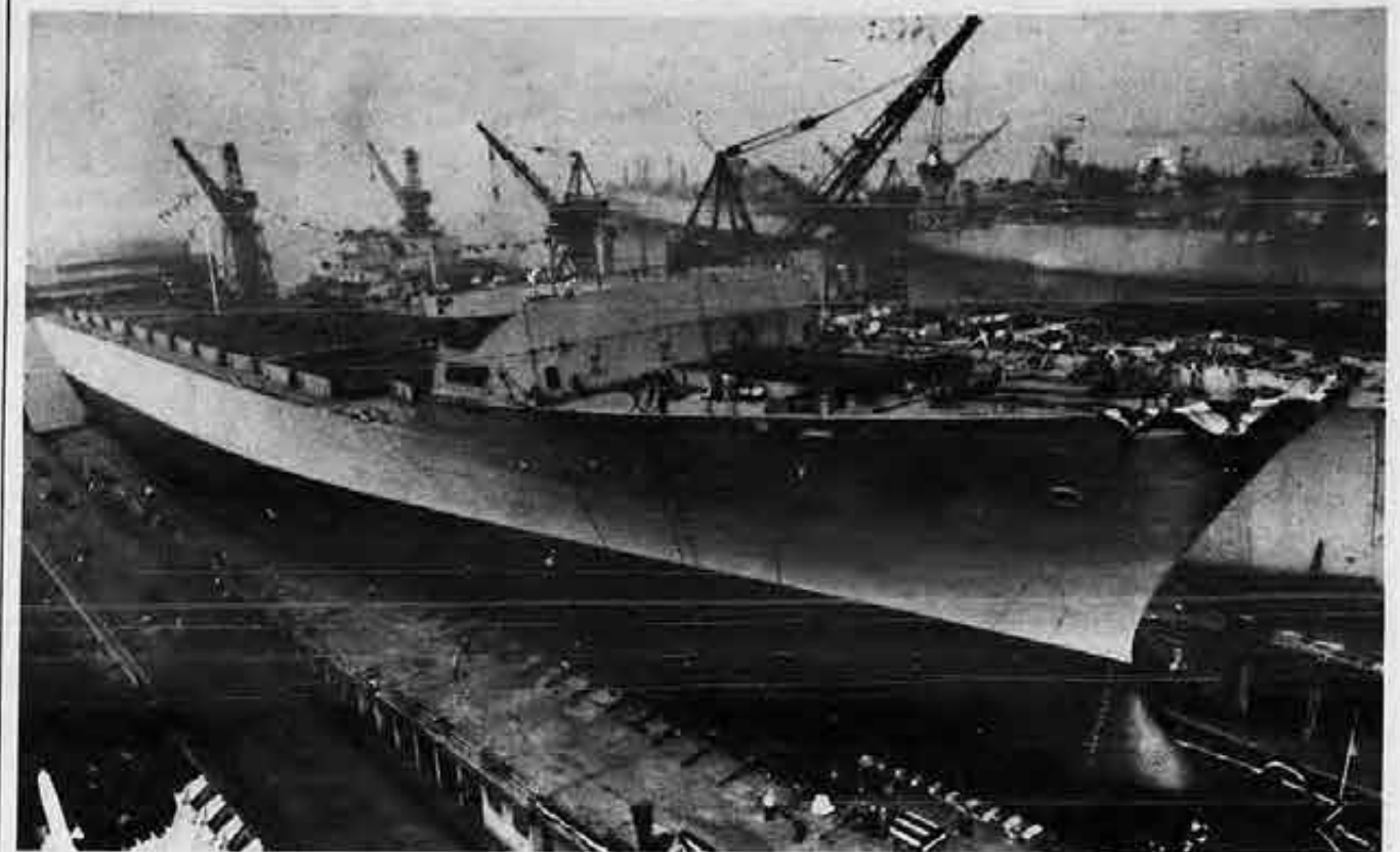
The Hawaiian Enterprise, a new 34,000-ton containership, was launched recently at the Sparrows Point shipyard. The SIU Pacific District-contracted vessel, which has a capacity of more than 1,000 24-foot containers, will be delivered to Matson Navigation Company in December. The 719-foot vessel will cruise at a normal sea speed of 23 knots, and is the first of two ships being built for Matson's Pacific service.
