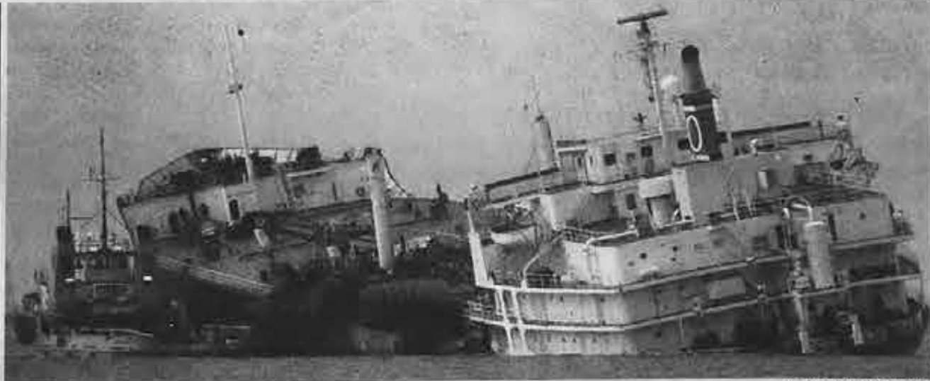
The 660-foot gasoline tanker OMI Charger lies with a giant hole in its side as a result of an explosion and fire that occurred October 9 near the mouth of the Houston Ship Channel close to Galveston, Texas. The cause of the blast, which killed three crewmembers, is under investigation.
