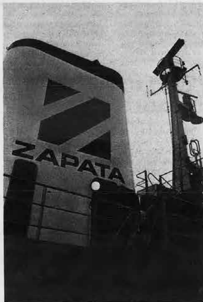
The smokestack and radar boom of the Zapata Rover .
