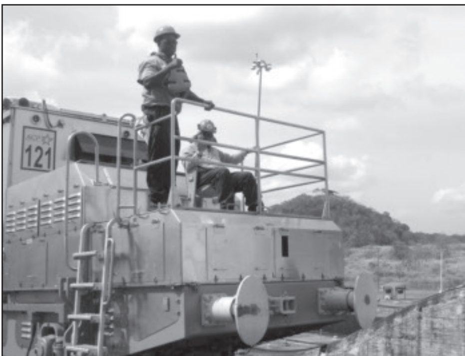
Members of the SIU-affiliated United Industrial Workers position their equipment (a railed locomotive called a Mule) into position to assist another vessel through the Miraflores Locks.
