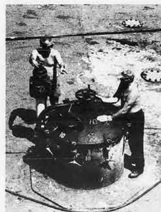
Francis McGaray, the bosun of the Erna Elizabeth tests the latch on Number 10 tank while David Berger lends a helping hand. All tanks aboard the ship were recoated during refitting.
