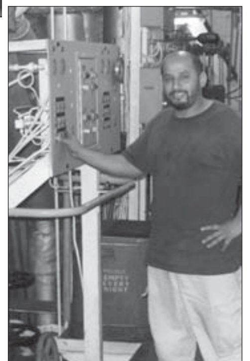
Abdul Rahman presses a button to blow the tubes. Rahman is the 4-8 oiler on the Horizon Spirit .
