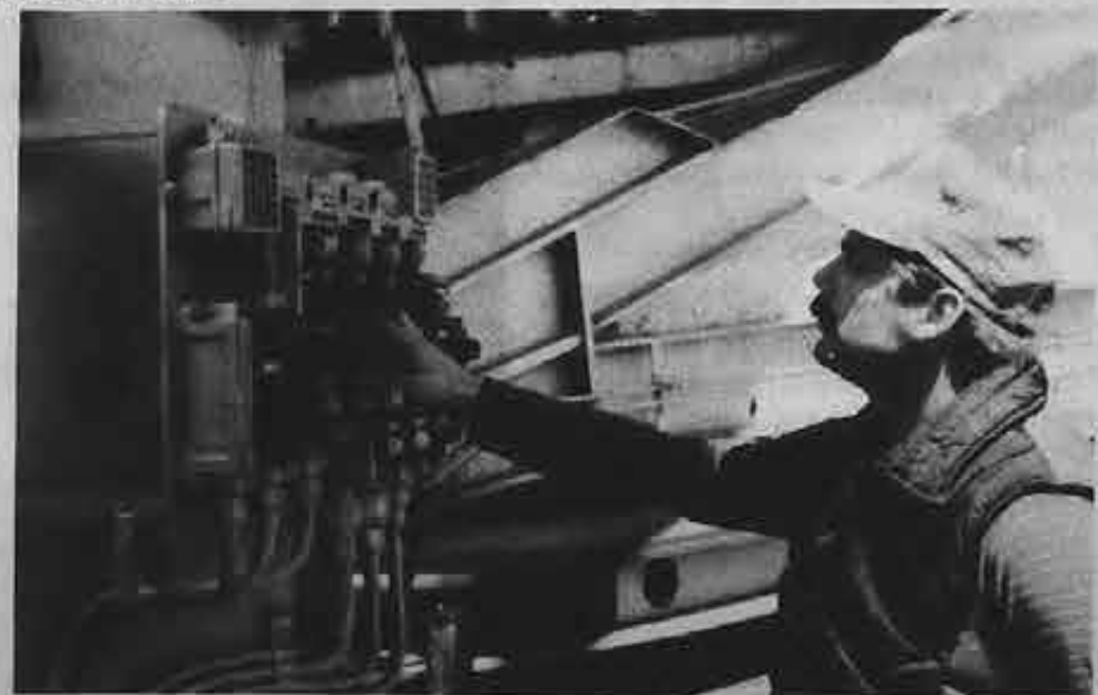
Conveyorman Norm Guild pushes the buttons to start the boom conveyor belt.
