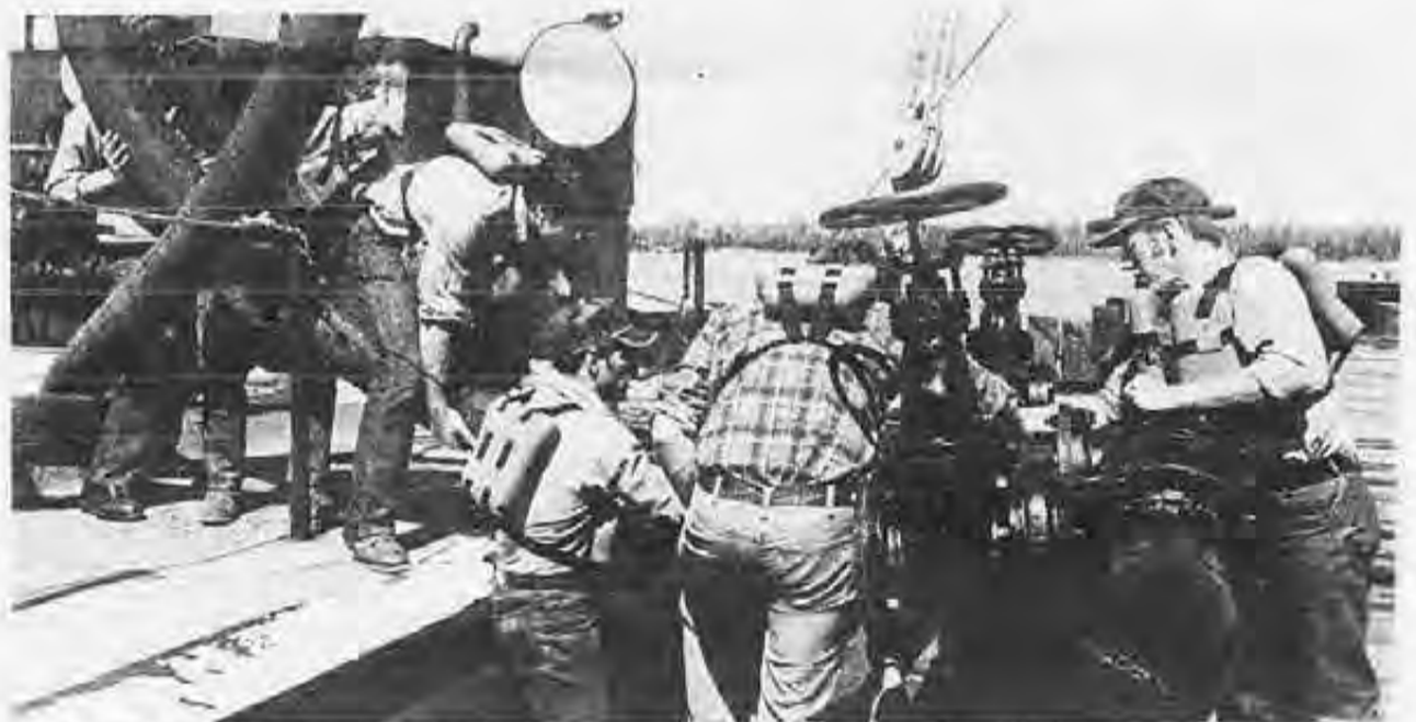
HLS trainees maneuver the cargo hose to secure it to the dock manifold. For these students, the tankerman course is a big step ahead in their career—when they pass the tankerman test, they qualify for the endorsement as soon as they complete the work time required by the Coast Guard.
