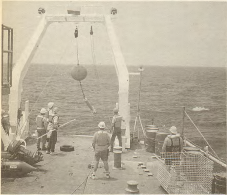
In the East China Sea, Seafarers recover current meter arrays which are used to conduct oceanographic surveys.
