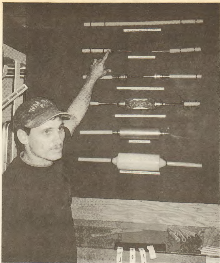
Several types of fiber-optic splices, shown above, are performed by Seafarers such as AB Splicer/Joiner Lyle Davis.
