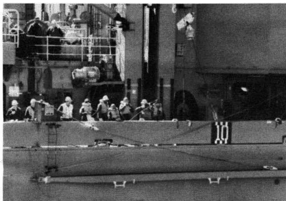
The first step in the cargo transfer maneuvers involves shooting a line from the Sylvania to the Southern Cross .
