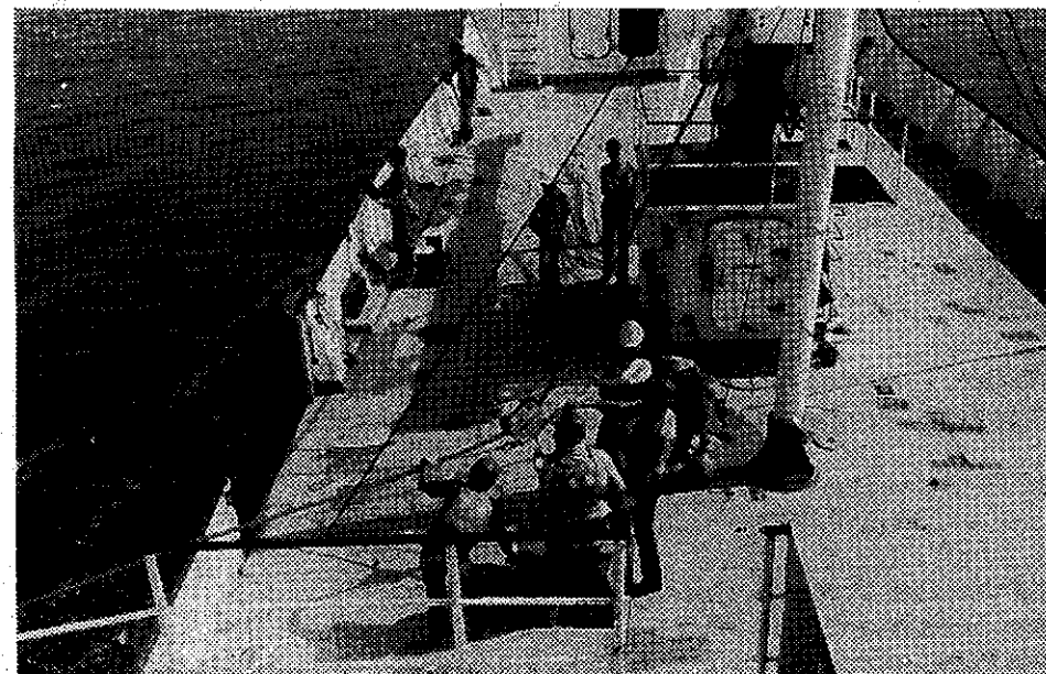
After the 5 inch manila highline is attached to the kingpost aboard the receiving vessel, a 55 gallon drum is prepared to be sent across.
