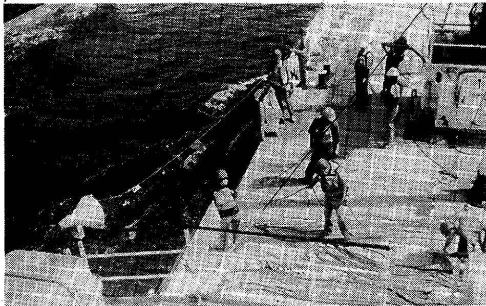
The phone and distance line is passed over to the receiving ship by means of the messenger line. A signalman, with colored paddles, coordinates the sending of the line, with his counterpart on the receiving ship.
