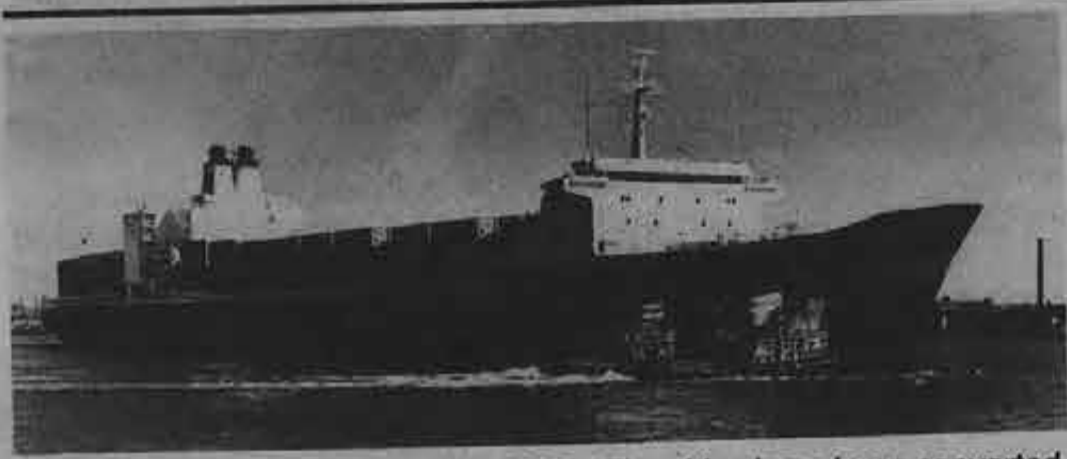
This is one of Sea-Land's former SL-7s. The ships have been converted for use by the Military Sealift Command in their Fast Sealift Ships program. Sea-Land, an SIU-contracted company, won the contract to operate the first four. Each ship will carry a crew of 26 unlicensed seamen.
