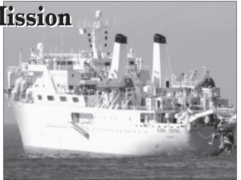
Photo by Todd Walsh, MBARI The Global Sentinel launches a plow used to bury cable beneath the sea floor's surface.
