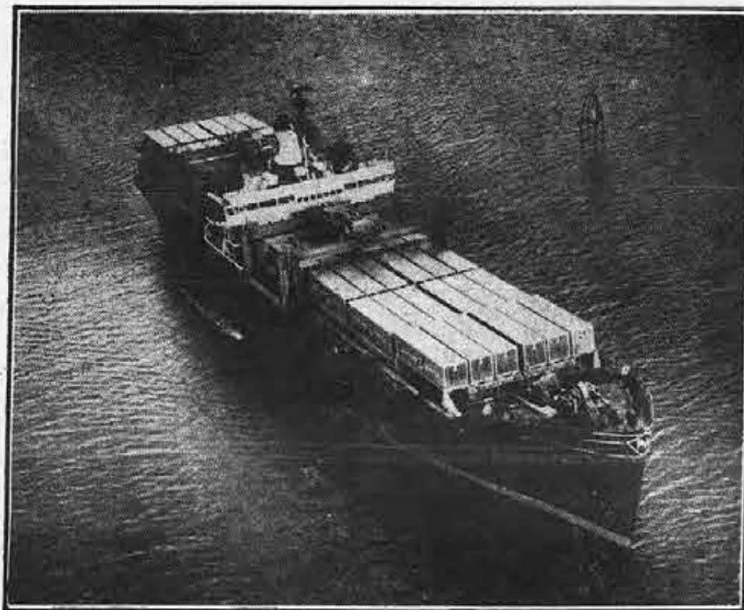
Fully-loaded ship shows radically-new deck gear. Note how entire crane body can move forward or aft on rails to any hatch.
