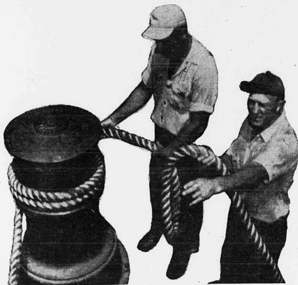
Handling lines is an old story aboard a towboat. Here SIU-Marine Allied Workers members Abe Bellande (left) and Robert J. Stoufflet, deckhands, take a hawser around a bitt on the DeBardeleben's deck.
