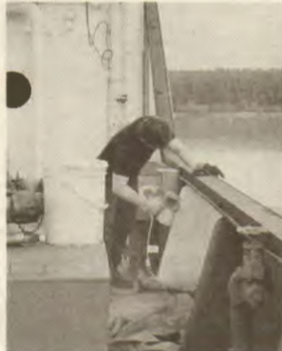
Painting bulwarks in a Toledo, Ohio shipyard is Deckhand Darren Lahaie.
