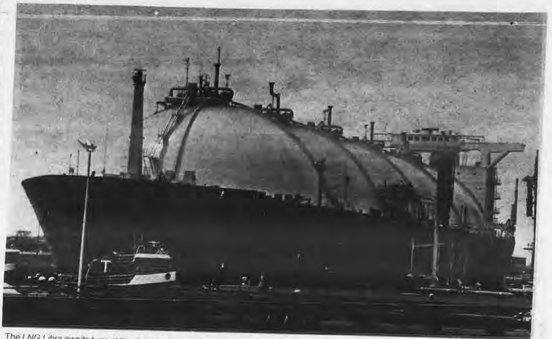
The LNG Libra awaits tugs at the dock in Everett, Massachusetts just prior to embarking on her maiden journey to Indonesia. The massive LNG carrier was here for cooling down of her tanks and to take on some LNG to use as fuel for the voyage.
