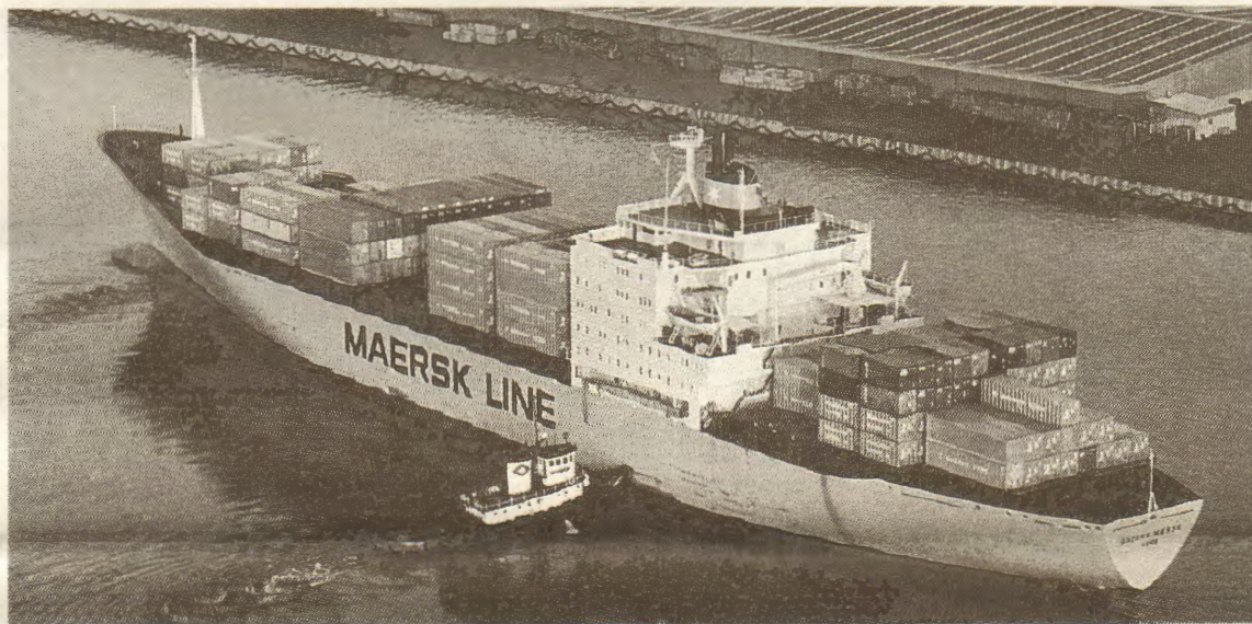
In this photo from 1976, the Swan Point , a Curtis Bay tug, assists the containership Anders Maersk , in docking with her starboard side to the pier in Philadelphia Harbor. The Maersk vessel is equipped with a bow thruster and a large bulbous bow. Notice the very streamlined and cutaway hull configuration, making it necessary for the tug to position itself more than 200 feet from the containership's stern.
