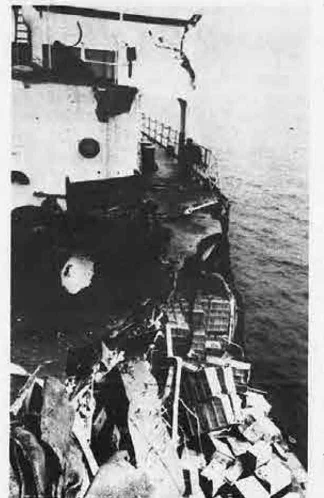
Impact tore away deck plates and smashed boxes of ammunition in ship's No. 3 hold. Complete story of Transpacific collision on page 3.
