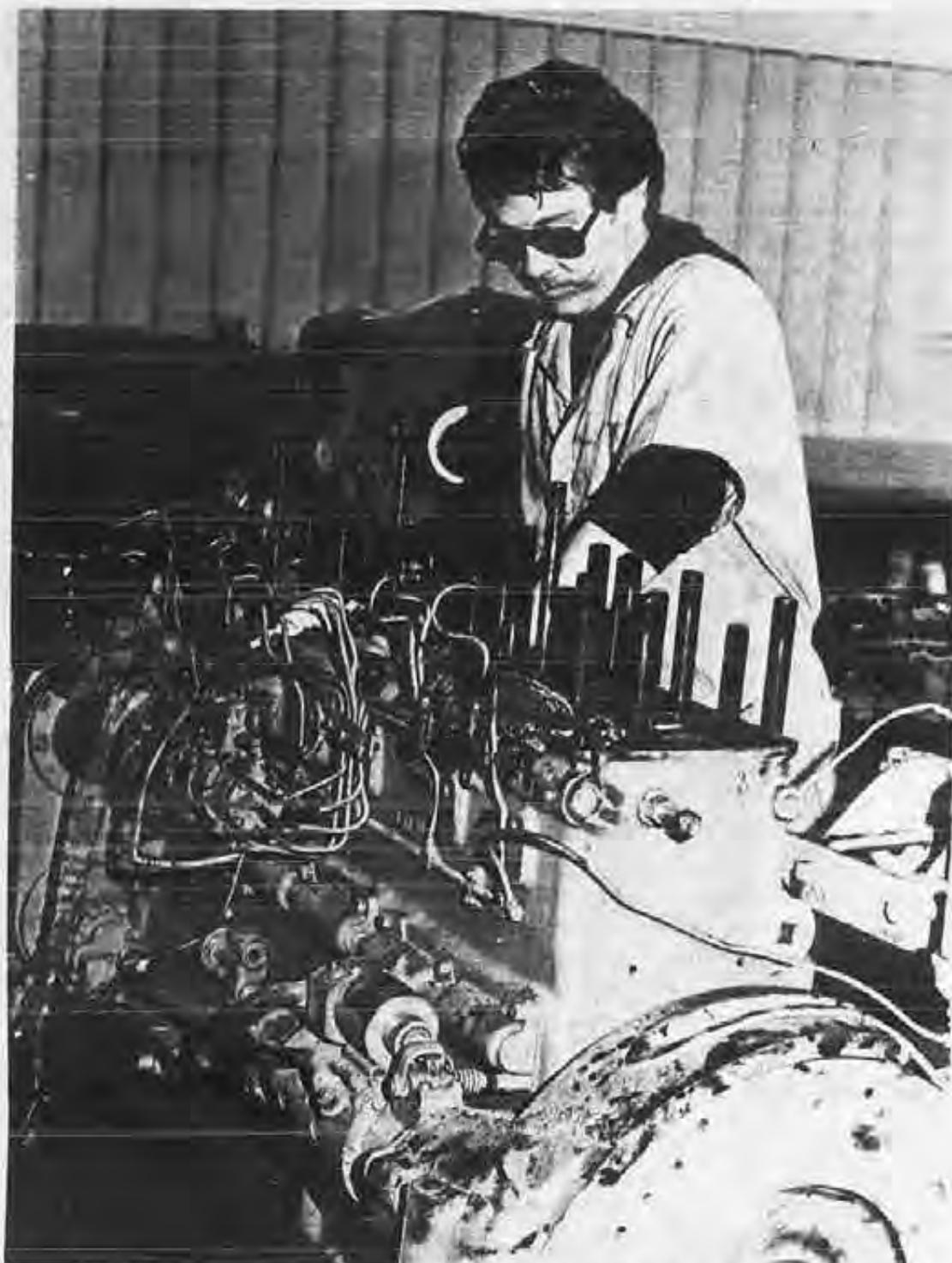
B. W. Morrison is shown in the HLS Machine Shop as he oils down the cylinder walls on one of the Lundeborg School's diesel engines.
