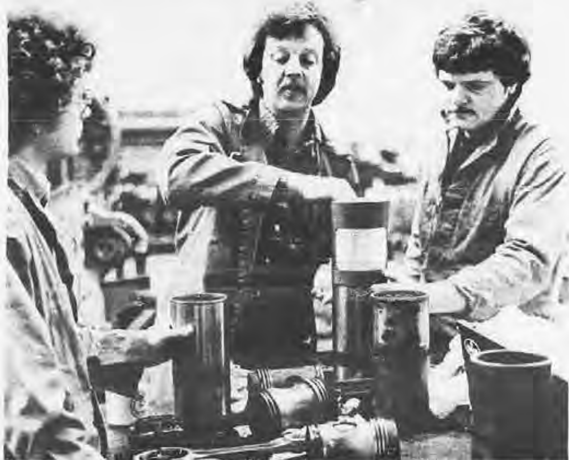
As part of their OJT, all the diesel engineering students practice compressing the rings on cylinders. Here, Bill Eglinton, the instructor, demonstrates this skill for James Redditt (left) and Ted Willms (right).
