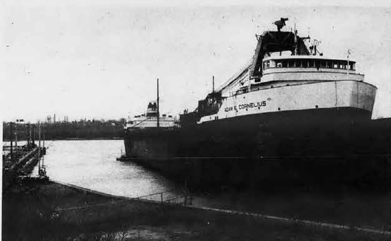
The Adam E. Cornelius, 666 feet long and 22,000 tons, gets her hull painted as she makes ready for her first trip of the year. The "Adam E." was the last United States bulk freighter built on the lakes. The big self-unloader came down the ways at Manitowoc, Wis., in 1959. She can carry 21,000 tons of coal, and unload in six and one-half hours.
