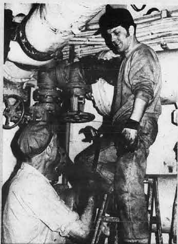
Monroe Daedler and Gene Hayes, oilers on the J.A.W. Iglehart, work on the oil cooler lines for the main engine as the ship is in final stages of fitout for the 1970 season on the lakes.
