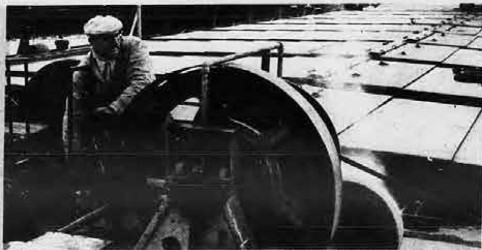
Ed Peterson, wheelsman, takes in on number 4 line, as the G. A. Tomlinson shifts astern at the coal dock in Toledo, Ohio. Working the two steam winches at the same time is tricky business, even for a veteran lakes Seafarer like Peterson.
