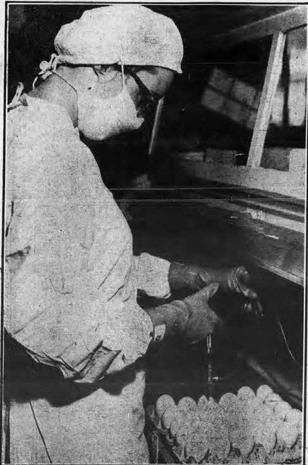
Drug manufacture is a major area of representation. Culture for a vaccine is prepared by injection into eggs.
