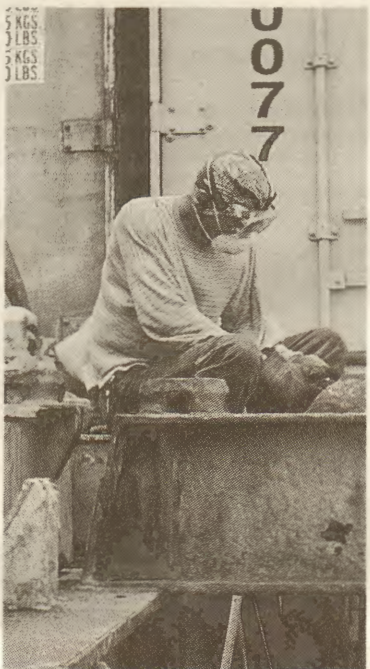
Chipping away old paint, as is being done by AB Jay Thomas (left) and AB Theodore Bush, is an important maintenance procedure.
