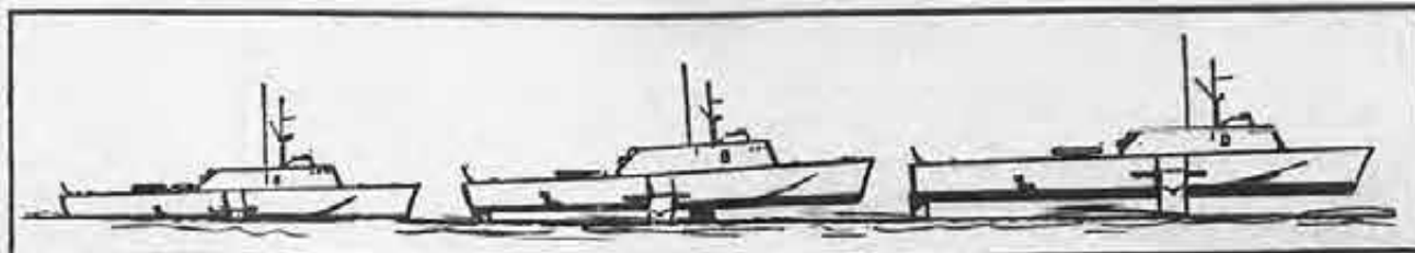
Artist's conception shows how the world's largest hydrofoil ship will "take off" from its normal displacement condition (far left) to its full foil-borne condition (right).
