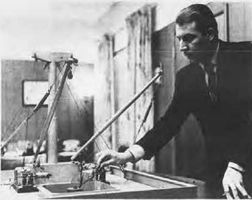
Raymond Liozzi, who attends SIU Deck Officer's School in New York, studies a working model that includes winches, lines, booms and handling gear used in the loading and unloading of cargo. Model is also used to demonstrate the correct way to get cargo into hold.
