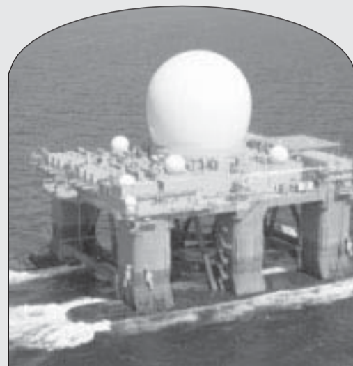
Seafarers sail aboard many different types of vessels, but the SBX (pictured at left) is one-of-a-kind within the SIU-contracted fleet. The semi-submersible craft—part of a U.S. operation called ground-based midcourse defense (GMD)—recently underwent modifications in Brownsville, Texas before sailing to Alaska. It is operated by Interocean American Shipping (formerly IUM) for the U.S. Military Sealift Command.
