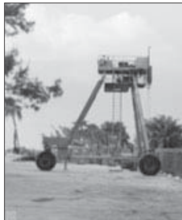
A Coastal Research Amphibious Buggy (CRAB) is a three-wheeled vehicle built by the Wilmington District of the U.S. Army Corps of Engineers to monitor beach nourishment projects.
