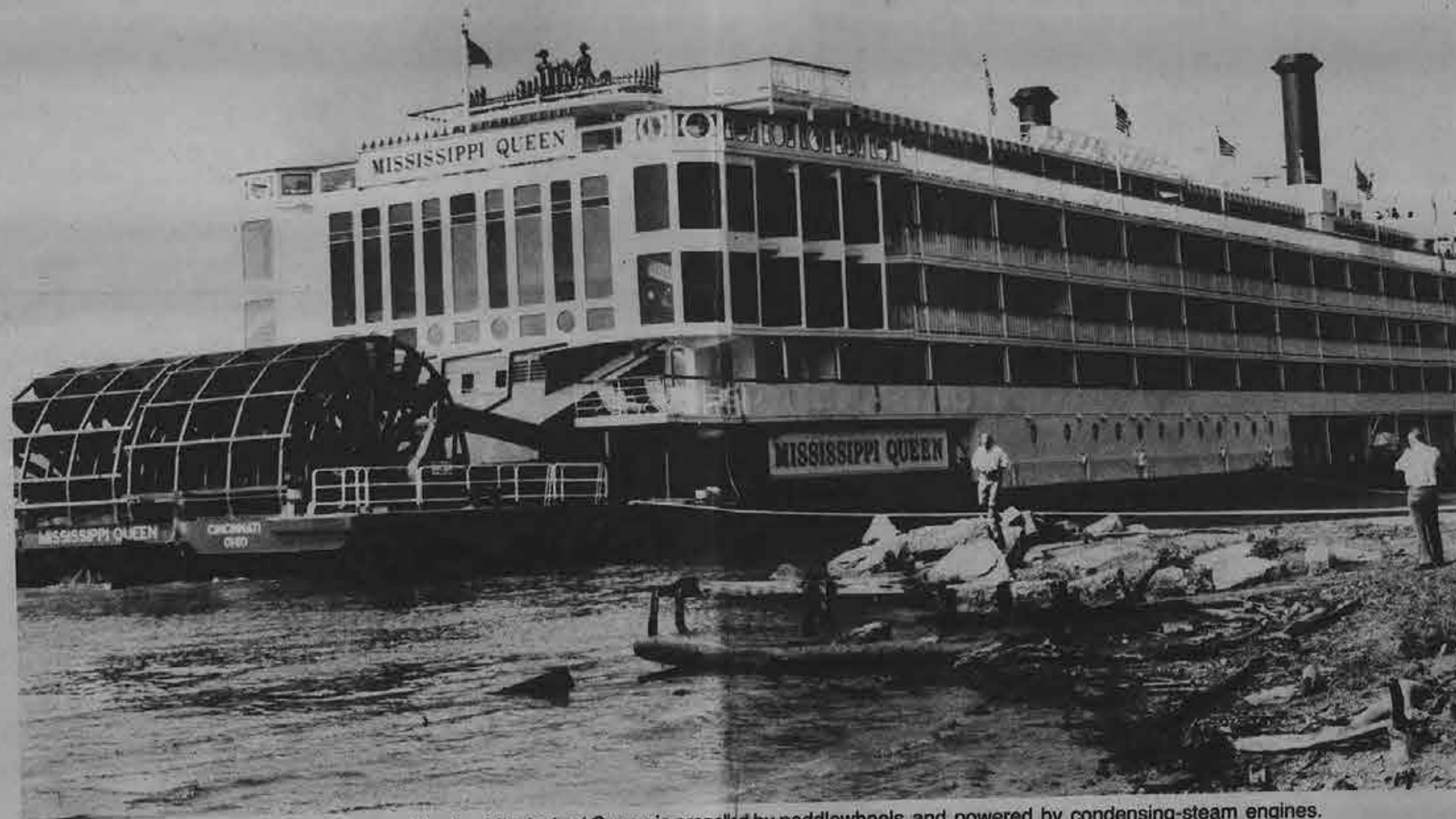
Considered a true steamship, the Mississippi Queen is propelled by paddlewheels and powered by condensing-steam engines. Each paddlewheel is 36 feet wide and 22 feet in diameter.
